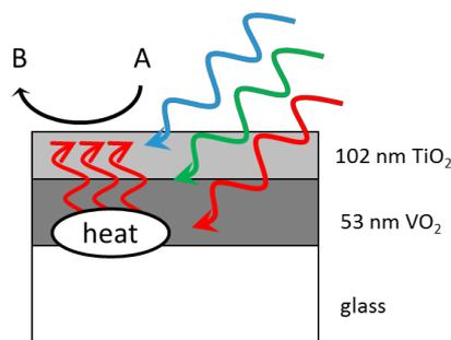
**Figure.1** Principle of spectral selective multilayer coatings with enhanced (i) photocatalytic activity, (ii) thermochromic and (iii) anti-reflective properties.
